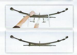
7. Wearing appropriate personal safety protection, use an angle grinder to trim the centre bolt leaving approximately 4 threads protruding through the nut and touch up the cut area with black paint to prevent rusting.
